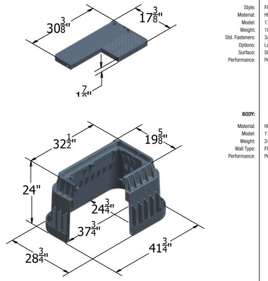
\*Cover comes standard with permanent markings for manufacturer, load rating, model size and manufacturing location.
